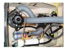
The Unit Has Easy Access to the Vacuum Motors and Pump Through a Suitcase Design
